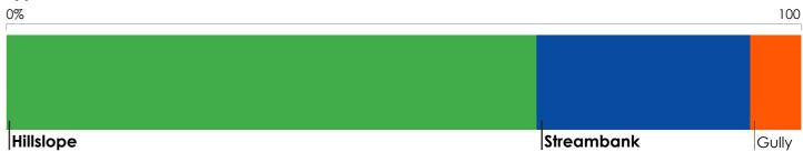
Most sediment erosion comes from hillslopes and streambanks in the Boyne catchment.
