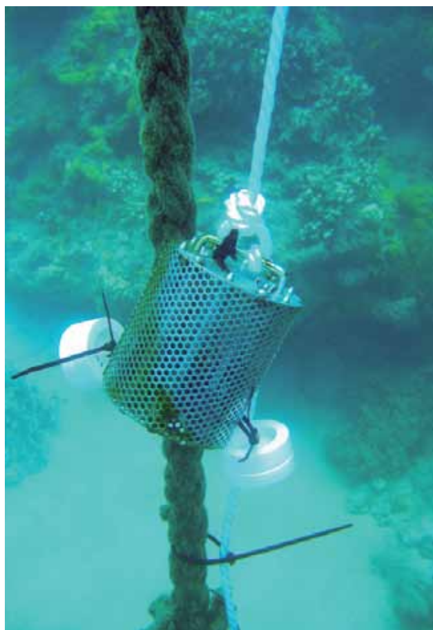
Figure 4.3 – Passive samplers monitor marine water pesticide concentrations (Image: J. Muller, University of Queensland).
